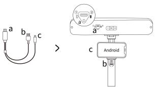
**Step 2**: Put a phone in the Phone Holder, and use the 2-in-1 Mobile Cable to connect to the ports shown. When the scanner's indicator ② turns solid green, it's powered.
