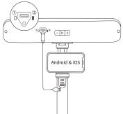
**Step 2**: Put a phone in the Phone Holder, and use the USB Type-A to C Cable or 2-in-1 Mobile Cable to connect the scanner to the Power Bank Handle. When the scanner's indicator ② turns solid green, it's powered.
