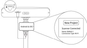
**Step 4**: Open Revo Scan, when the software shows Scanner Connected (iOS devices will show the scanning preview window) and the scanner's indicator ① turns solid blue, it's ready.
