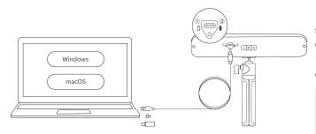
**Step 2**: Use the USB Type-A to C Cable to connect the scanner to a PC. When the scanner's indicator 2 turns solid green, it's powered.
