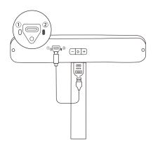
**Step 2**: Use the USB Type-A to C Cable to connect the scanner and Power Bank Handle. When the scanner's indicator ② turns solid green, it's powered.
