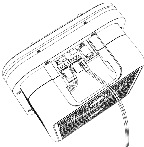
or External power supply 24V (Double check the polarity)
