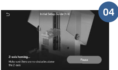
Wait for the Z-axis lifting
