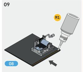
The areas where the glue should be applied are marked in yellow. Make sure that you only use a thin layer, otherwise the adhesive will run out of the joints and the adhesive residue will not look nice on the model.
