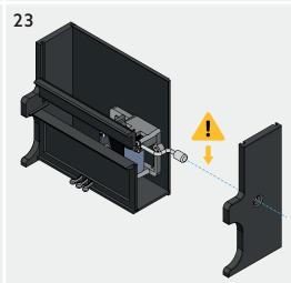
Once the handle has been threaded in, make sure that the lid mechanism is inserted into the correct position of the side panel when attaching the side panel.
