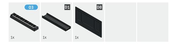
Slide the keyboard from step 03 into the keyboard bay D1.
