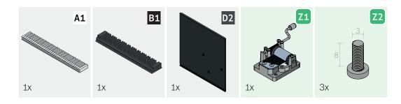
Insert the white keys [A1] into the black keys [B1]. Hold the white keys at an angle to make it easier to insert them into the black keys. Press at the rear end of the white keys to secure them in place.
