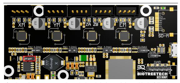
2) When using USB to power the motherboard: the jumper is inserted in the following "VUSB" position
