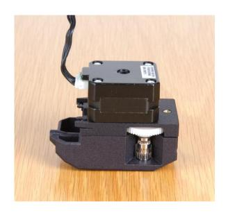
Mount the stepper motor into the extruder rear.
