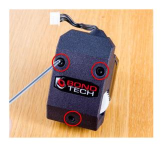
Carefully tighten the three M3 screws.
