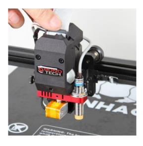
Disconnecting the flatcable to the printhead and put it out of the way
