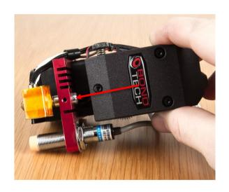
Slide the extruder onto the bottom plate guiding the recess for the heat break so it fits over the heat break, align the two M3 bottom holes with the screws removed earlier and tighten them using a 2,5mm hex wrench.
