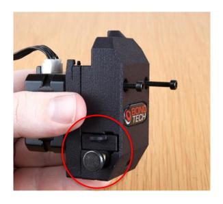
Align the stepper motor and extruder bodies together and insert the two M3x30. Insert the hinge and thumb screw back into its slot.
