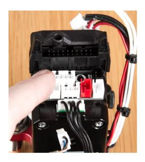
And then press the board downwards until it clicks into place. Take it carefully and make sure it is in the correct position before it is pressed down.
