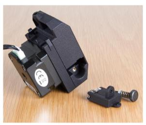
Remove the thumbscrew and hinge from the extruder body.
