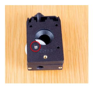
Take the new part and carefully assemble the extruder bodies together and make sure the gear shaft is correctly placed inside the bearing.
