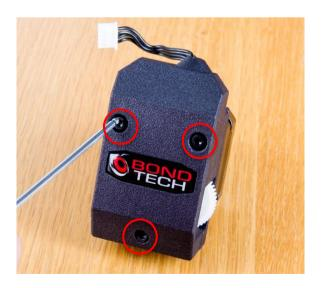
Loosen and remove the 3 M3 screws clamping the motor and extruder together using your 2.5mm hex wrench.
