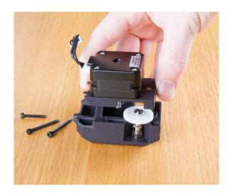
Place the extruder with the Bondtech logo face down and remove the motor and rear from the extruder body.
