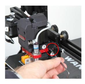
Use a 2.5 mm hex wrench and loosen the two screws on the right that hold the extruder assembly to the carriage.
