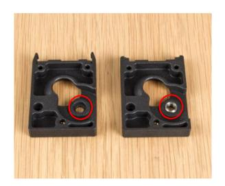
Remove the 5 mm bearing from the old part and assemble it into the new.
