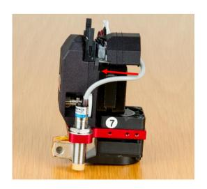
Slide the new cover over the board, make sure to arrange the cables so it fits into the cut-outs on the left side for the wires to the cooling fans and the hotend.
