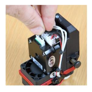
Remove the break board cover and loosen the connector to the stepper motor carefully.
