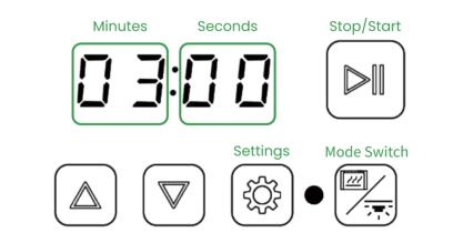
3 Select to start curing and drying, or select or select again to confirm the curing time
