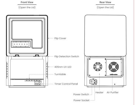
D282 mm x H162 mm 8000-10000 μW/cm² Multifaceted UV Light (A total of 24 UV light beads) Heated Drying 360° Rotating Curing 45±3°C (Affected by ambient temperature) Drying: 0-15 minutes (Default: 3 minutes);
