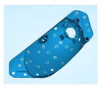
**Watertight:** When the scan is completed, click , proceed to post-processing. You will see two modes after clicking the button, as shown in the picture:
