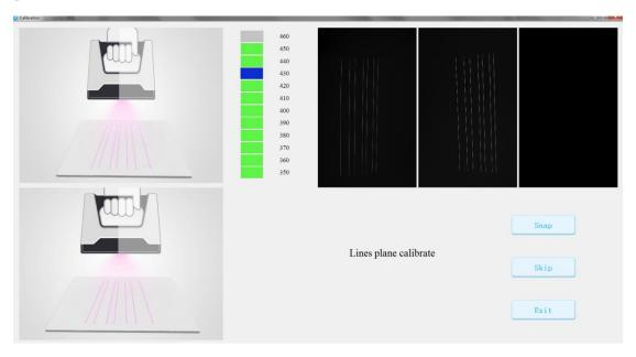
When the distance bar appears all green, the software starts to calibrate automatically. It will show "HD calibration success" when calibration is finished. If there is no color camera, click "Exit" to exit the calibration page, enter the scan mode selection page.
