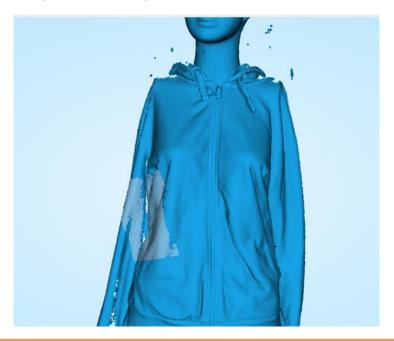
If the merger fails during the scan, please go back to the scanned part for 3 seconds where there are features and details, start to scan again when it is followed again.
