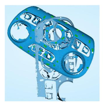
Click button to open Manual Align view port on the left side of the software. Keep SHIFT down, and click left mouse button to select at least 3 non-collinear corresponding points in the 3D preview windows for Manual align.
