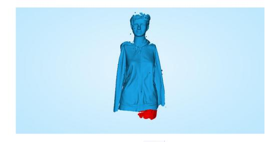
**Watertight:** When the scan is completed, click , proceed to post-processing. You will see two modes after clicking the button, as shown in the pictures:
