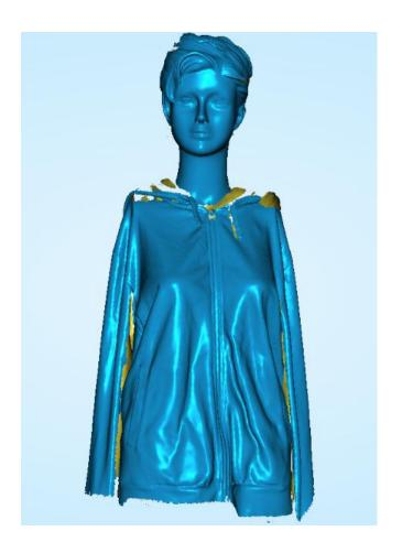
: Watertight for print: Closed model can be printed directly. You will see the pictures pop up as following after selecting this encapsulation. Select the object details.
