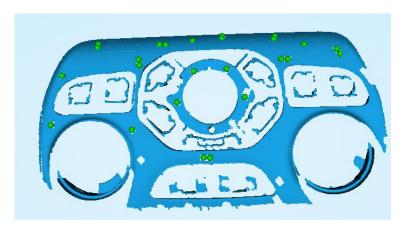
When the edition is completed, change the position of object or scanner for next scan. If use feature align, make sure the overlap area of currently scan area and the last scanned data is
