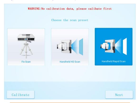
Note: Scanning can not be entered if calibration is not done. Please do the calibration first when there is a WARNING: No calibration data, please calibrate first.
