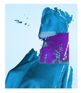
You need to go back to this scan data position and wait for about 3 seconds or find the previous scan data position with features and adopt merging features for about several seconds, and then try to scan normally.
