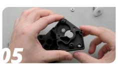
Place the new ball bearing into the rear part of the body.
