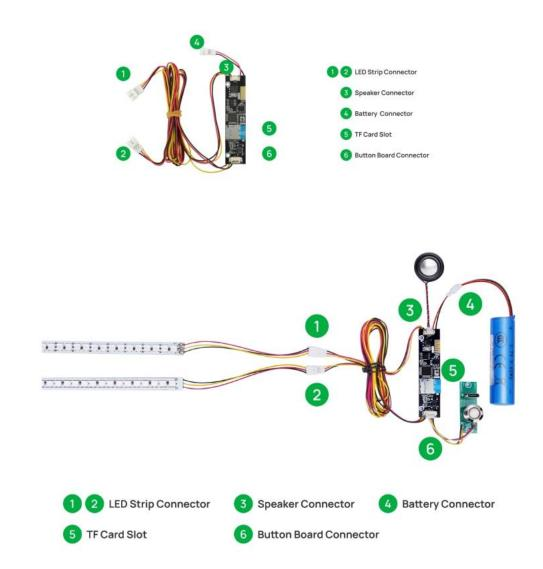
3. Perform a function test on the internal structure module: After connecting the two LED strips, turn on the power and check whether the lighting and sound effects are working properly. If the power doesn't turn on, charge the internal structure module first and then retest.
