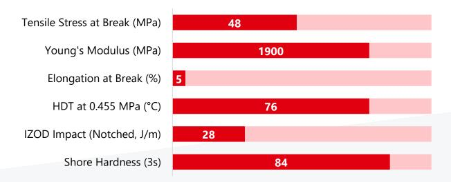
\*Values shown are linked to parts printed on a DLP printer at 385nm & post cured with broad spectra bulb (Loctite UVALOC 1000)
