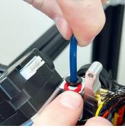
The printers original Bowden tube will be reused to help guide filament from the spool into the Extruder
