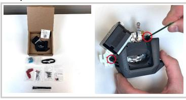
Prepare the NG extruder for assembly by removing the fan shroud
