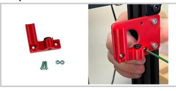
Install the filament guide bracket where the original Bowden extruder used to sit, using provided M3 nuts and bolts
