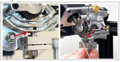
• Insert the hotend assembly into the extruder
