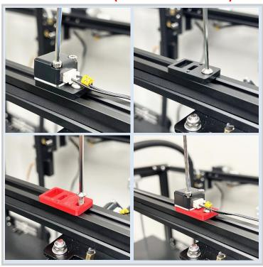
The x-axis endstop switch needs to be moved to the left (Only on Ender 5 Plus)
