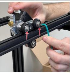
Insert the provided <u>shorter</u> M5 screws into the two remaining V-Roller wheels
