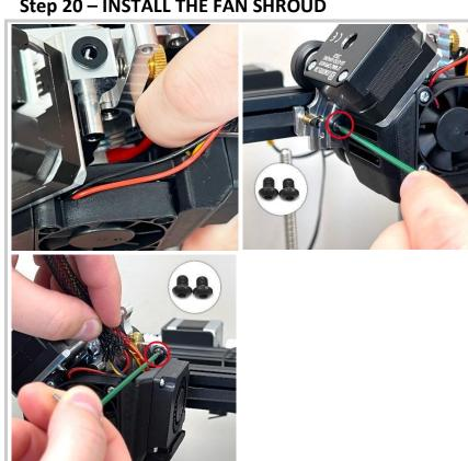
Install the assembled fan shroud back on the extruder
