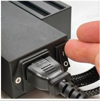
• Plug the power cable in and turn the 3D printer on
