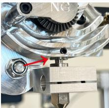
Verify that the thermal break is seated as deep as possible inside of the extruder (compare with reference image on the left)
