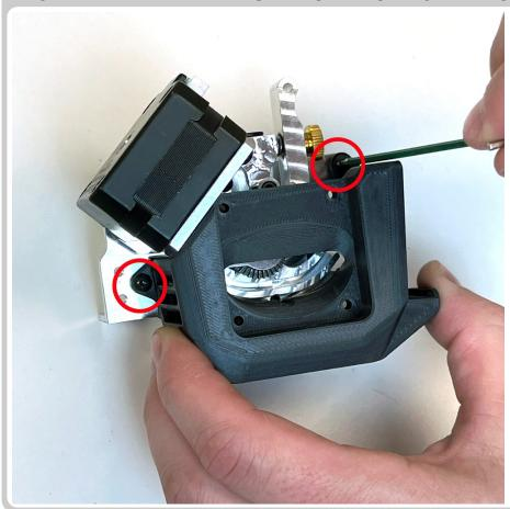
• Prepare the NG Extruder assembly by removing the 3D printed fan shroud
