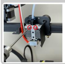
• Remove the two screws holding the hotend on the carriage plate (2.0mm Allen wrench)
