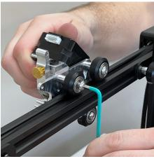
• Insert the shorter two M5 screws into the two remaining V-Roller wheels
