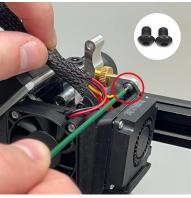
• Re-attach the fan shroud to the extruder using two screws (2.0mm Allen wrench)
