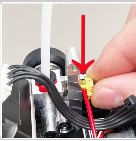
• Adjust the drive gear tension by rotating the brass knob
