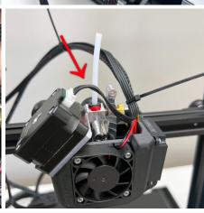
Use the custom extension cable provided with the NG kit - it has the special wiring pinout that is required to connect the LDO motor to a Creality 3D printer
