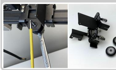
• Remove the M5 screws and nut holding the three V-roller wheels
