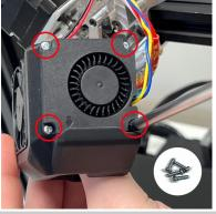
• Attach the hotend cooling fan to the front of the 3D printed fan shroud using the larger self-tapping screws provided with the kit
