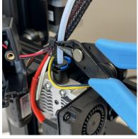
• Remove the single M3 screw holding the fan shroud in the back of the carriage plate
