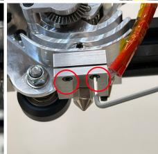
• Insert the heater cartridge and thermistor into the heater block
