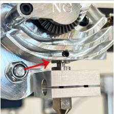
• Attach the hotend assembly to the extruder
