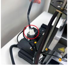
Use the custom extension cable provided with the NG kit - it has the special wiring pinout that is required to connect the LDO motor to a Creality 3D printer
