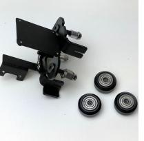
• Remove the M5 screws and nut holding the three V-roller wheels
