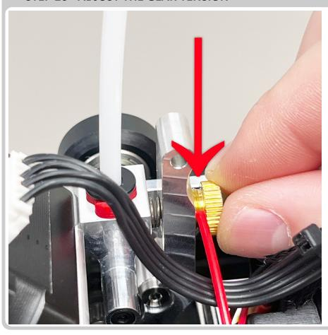
• Adjust the drive gear tension by rotating the brass knob
