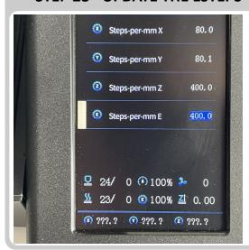
• Change the Esteps to 400 and save the setting by navigating the 3D printer screen menus to:
