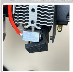
Make sure the hotend is at room temperature before touching the heater block
