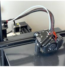
• Using the provided M3 screws and nuts, attach the 3D printed PTFE bracket to the mounting holes which previously held the stock Bowden extruder
