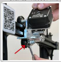
• Adjust the eccentric nut on the bottom wheel to eliminate any carriage wobble (10mm spanner wrench)
