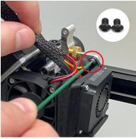
• Re-attach the fan shroud to the extruder using two screws (2.0mm Allen wrench)
