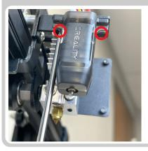
• Remove the two screws holding the CR-Touch (2.0mm Allen wrench)
