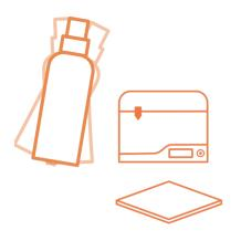
1 - Shake the bottle well for 5seconds and take the printbed out of the 3D Printer. Remove any left residue from previous prints. Every component should be at roomtemperature.
