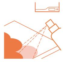
2 - From a distance of 10cm or 4" apply PrintaFix Basic in overlapping circles on the printbed. Avoid uncovered areas that could effect the adhesion. Let it dry for 30sec.
