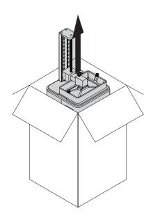
Take the printer out of the box. Don't grab the Z-axis screw when lifting the printer.
