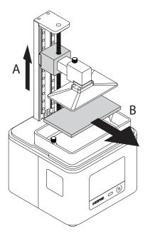
Move up the platform by gripping the platform block and pulling it upward (A). Remove the cushioning (B).
