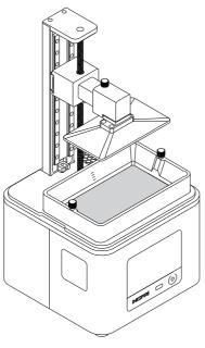
Clean the FEP film inside the resin tank with a cloth.
