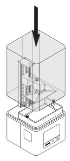
Remove the foil from the UV cover. Install the UV cover on the printer. Place the cover's seam behind the Z-axis.
