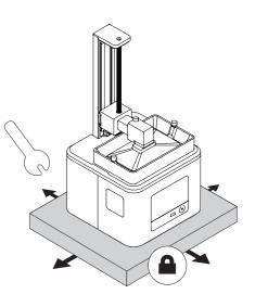
Place the printer on a flat and stable surface. If the printer remains uneven, use the plastic wrench from the Starter Kit to tighten or loosen the printer's legs as needed.
