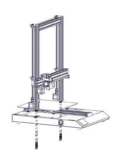
Step 5 Connect the Z Stepper Motors as shown in the pictures below:
