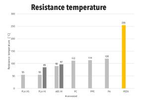
The resistance temperature is a value for the maximum operating temperature. Note, the closer you get to this value, the more the material properties change. When working at the limit we recommend checking exactly, if the material is suitable for the use case.
