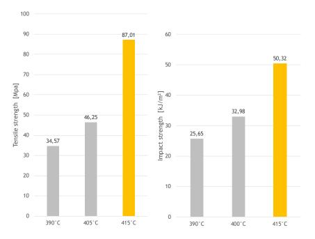
The printing temperatures have a major influence on the material characteristics. For high tensile strength and high impact strength, nozzle temperatures of about 415° C are required. The specimens were printed with simplify3D on a Creatbot F160 printer with 130° C heating bed and a closed printing chamber at the xy plane.
