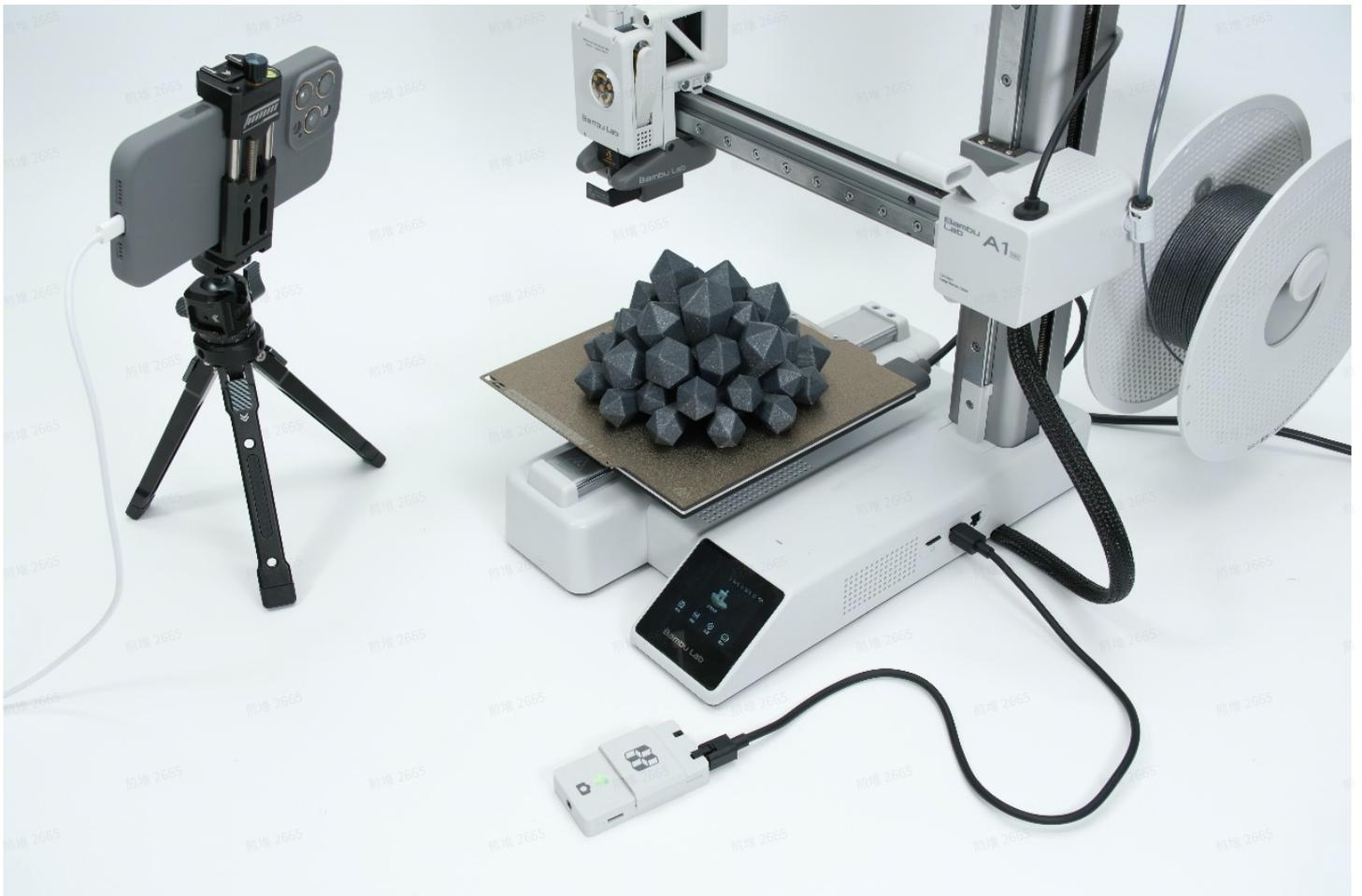
2. Place the phone in front of the printer. For A-series models, leave space for the heated bed to move, preventing collisions with the phone.
