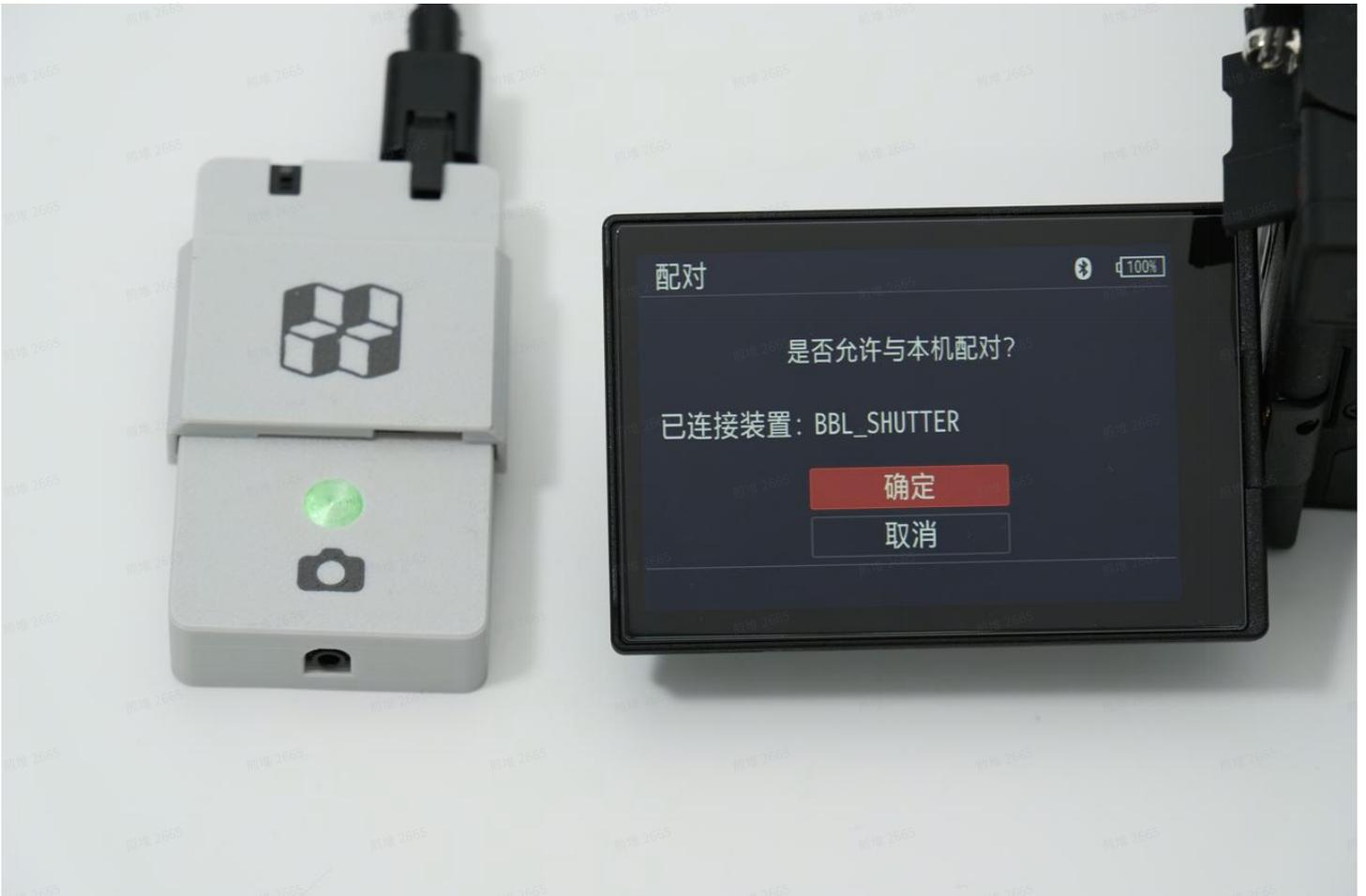
4. If the camera cannot detect the kit, disconnect the kit from the printer for 2 seconds and reconnect it. Ensure no other devices are interfering with the Bluetooth pairing port.
