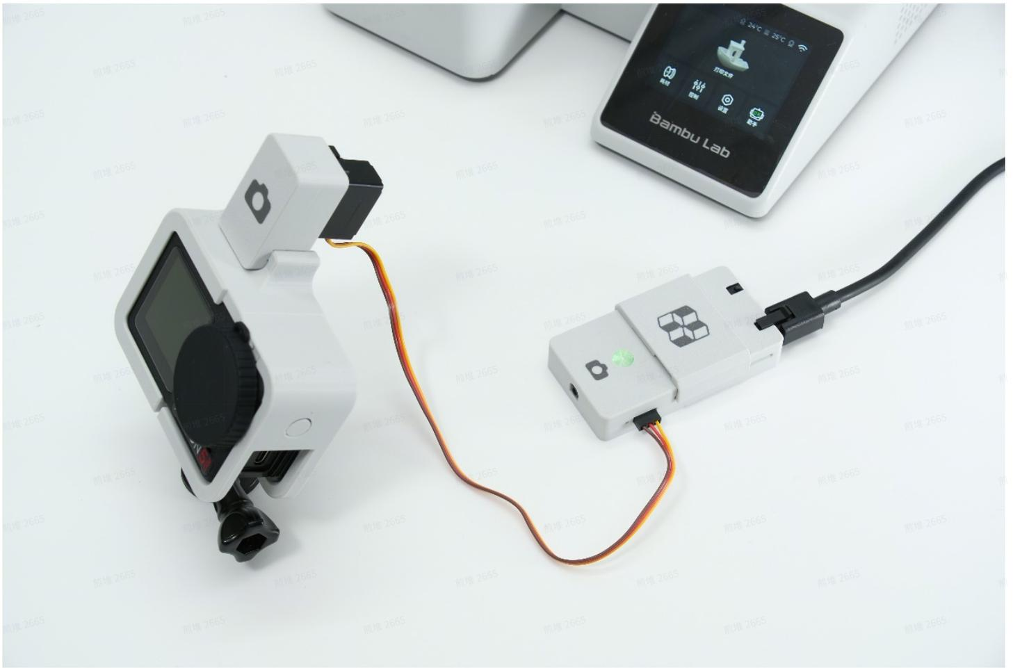
2. When using the servo shutter, manually modify the G-code to increase the shooting delay to 1000ms and enable the use of a purge tower.
