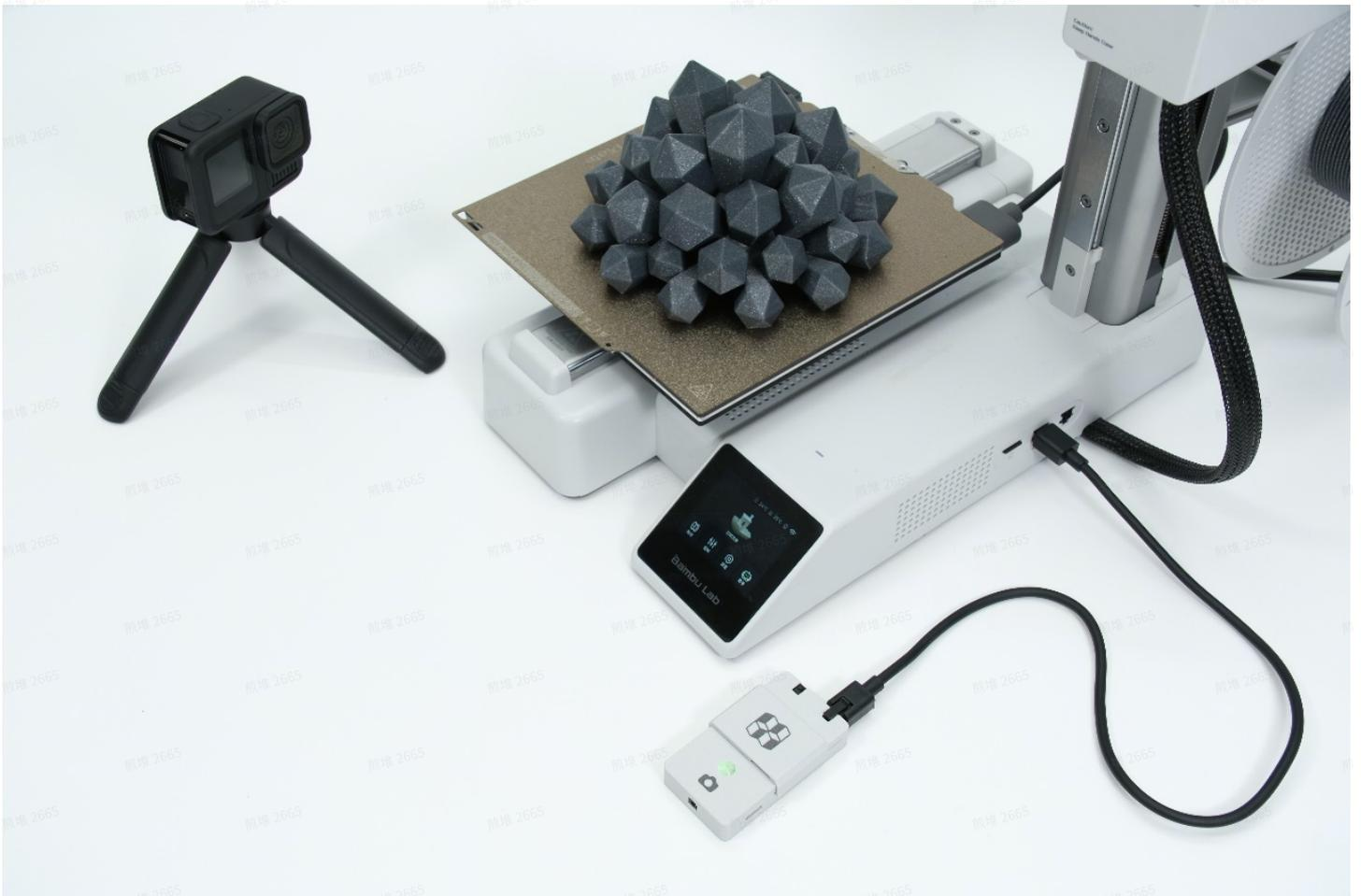
1. Connect the GoPro HERO13 to the timelapse photography kit via Bluetooth. Increase the auto-lock screen time in the GoPro settings to prevent the screen from locking during shooting. Since the shooting duration is long, connect the GoPro HERO13 to a charger.
