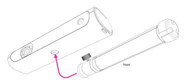
Connect the tripod to the scanner body by inserting the screw thread on the top into the screw hole in the another and tighten it clockwise as shown in the picture.
