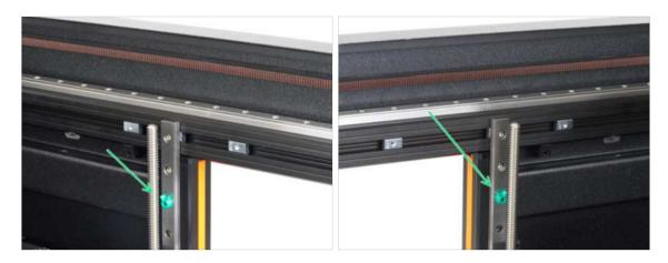
Take off the linear rail stoppers on both inner sides of the printer.
