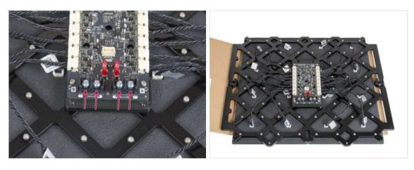
Remove the four power terminal screws using the Phillips screwdriver. Keep them aside as we will need them in the next step.
