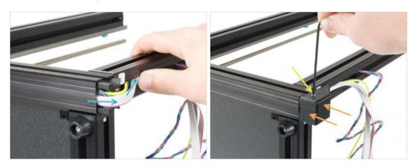
• Gently bend the cables over the corner and insert them into the extrusion. Start with the Z motor cable and then proceed with xLCD and PE cables. Gently bend the xLCD cable over the corner and insert it in the extrusion.
