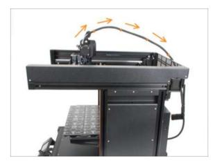
• Guide the extruder cable bundle with the PTFE tube freely over the printer to its rear side.
