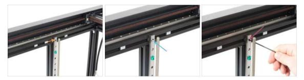
On the left side of the CoreXY, there are three M3nEs nuts in the extrusion. Slide the middle M3nEs nut behind the linear rail. Align its hole with the hole in the linear rail.
