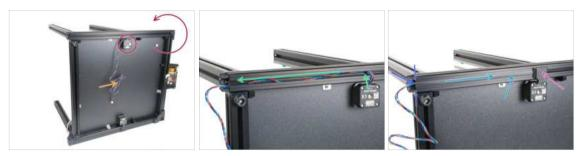
• Turn the printer so that you have the second motor on the top side.
