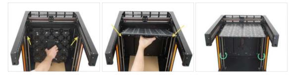
• Take the Heatbed and attach it to the top of the threaded rods. Both of the trapezoid nuts on the sides must engage onto a threaded rod.
