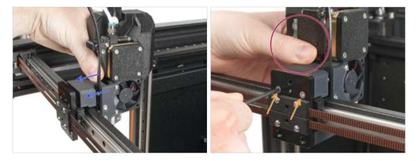
• Attach the extruder assembly to the X-carriage. See the correct orientation of the extruder.
