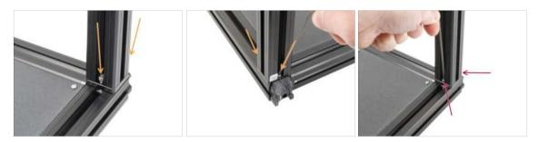
Insert two M4x12 screws, from opposite sides of the extrusion.
