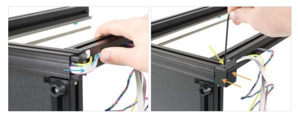
Gently bend the cables over the corner and insert them into the extrusion. Start
