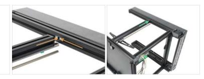
Be careful while attaching the extrusions and CoreXY, avoid scratching them.
