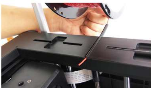
7. Insert the filament into the filament guide.
