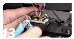
Cut the zipties securing the wire loom coming from the toolhead.
