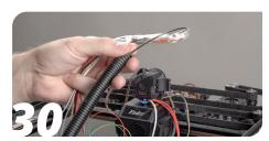
Push and pull the wiring loom through the conduit.
