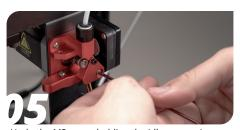
Undo the M3 screw holding the idler arm using a 2.5 mm hex key, then remove the idler arm.
