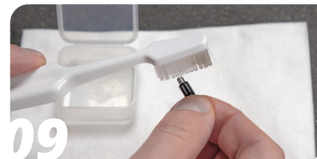
Dip the toothbrush in the alcohol and brush the needle bearings while on the pins
