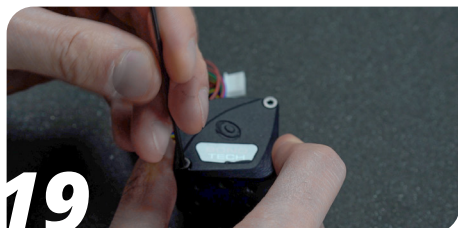
Add the two M3 screws and tighten with a 2mm hex key
