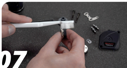
With a toothbrush, clean the gears
