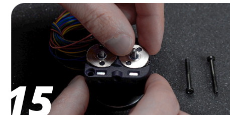
With the lever in the leftmost position, insert the drivegears
