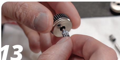
Place the lubricated needle bearings and pins in the drivegears
