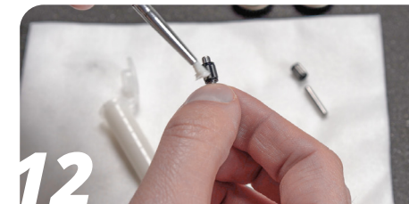
Using a small brush and our PrintSmooth grease, lubricate the needle bearings
