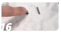
Insert the pins with needle bearings in the drivegears.
