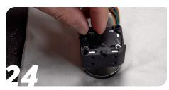
Add the lever to the drivegear pin.
