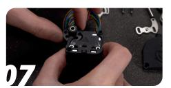
Lift the needle bearings out with your 2 mm hex key.
