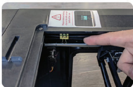
8. Remove the belt fixing clip of the right Y-axis.
