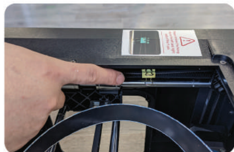
9. Remove the belt fixing clip of the left Y-axis.
