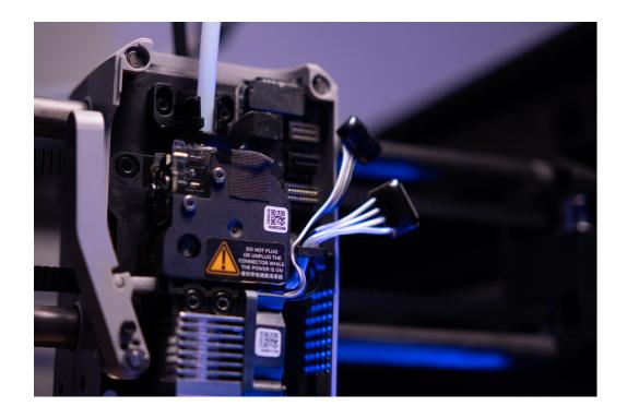
**Step 4:** Plug in the the hotend fan and the heater connectors to the board
