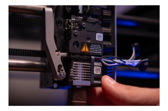
**Step 2:** Gently push the 2 screws in and then tighten them equally, be careful not to over-tighten
