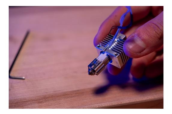
**Step 5:** Apply grease to the thermistor and the thermistor hole. Then, insert the thermistor into the hole in the side of the hotend and slide the retaining clip over it all the way up.
