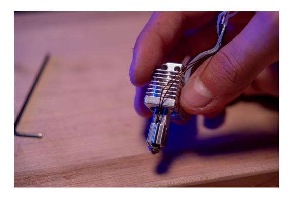
**Step 6:** Route your wires through the designated slot of the heatsink and be sure to place the thermistor wires behind the heater wires and slide the air dam over the wires.
