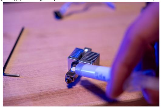
**Step 2:** Insert the heater adapter by sliding the ears of it into the top of the hot block
