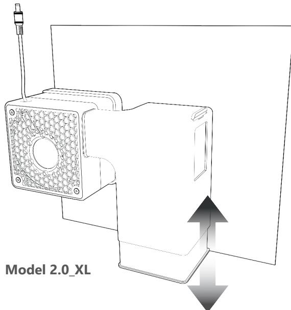
XL version – vertical snap-fit: to remove/install the bin, press in vertically.
