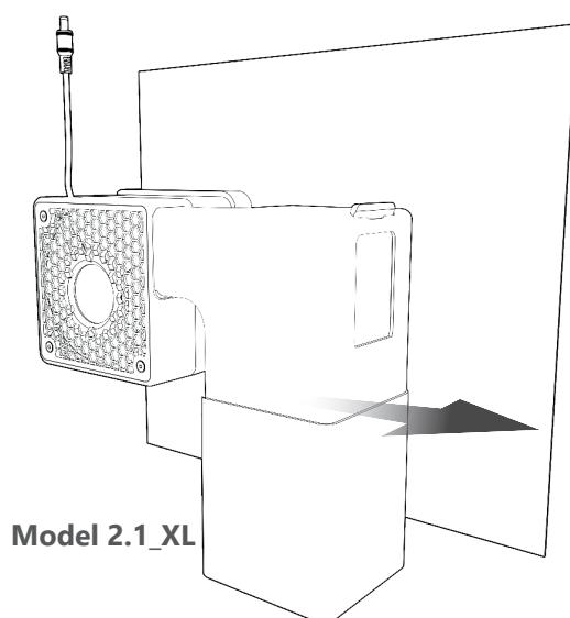
XL version – lateral slide: to remove/install the bin, slide it sideways.
