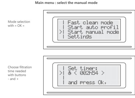
To reset the tiemr to zero faster, press buttons - and + together in the same time.
